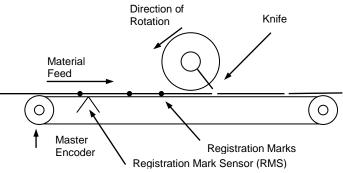
In the case where the RMS stops detecting registration marks (i.e. material is not present), the knife comes to a stop after the Cut Segment. Once a mark is read, the knife starts back up again to get into position for the next cut.
