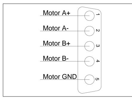
The "Motor GND" signal is connected to the controller chassis. This pin should be connected to the shields and shield drain wires associated with the two driver twisted pairs. It should be connected at both the controller and motor ends of the cable, also connecting to the connector housings at both ends.
