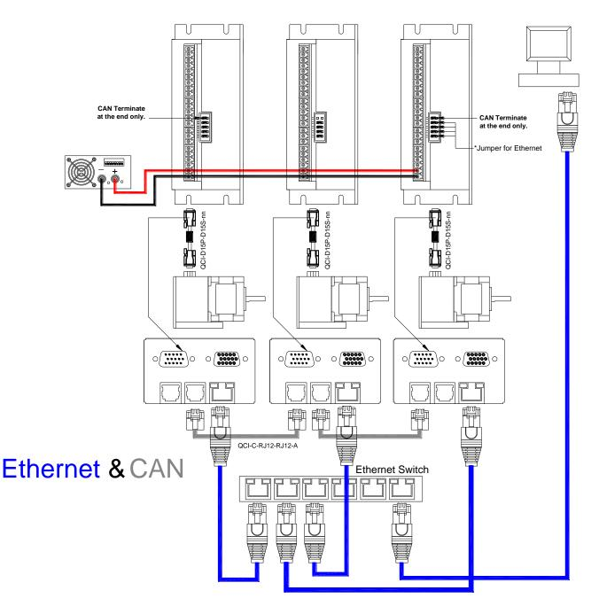
The above configuration shows a three-axis system with each axis having its own E-485 Bridge. CAN is configured as an inter-axis communications network to provide coordination and data sharing between the axis through QCI-C-RJ12-RJ12-A cables. Each axis has a unique IP address (for Ethernet) and a unique Unit ID (for CANopen). The router/switch provides communication between the PC and all of the SilverDust units. See Technical Document "QCI-TD056 E-485 Bridge-Ethernet".
