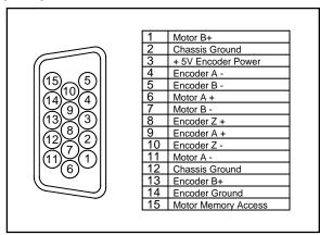
QCI recommends our QCI-C-D15P-D15S-nn (nn = length) cable to interface between the motor and the controller. Note: 01, 02, 04, and 10 foot cables are standard lengths.
