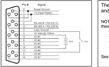
These signals provide power, communications and 3.3v IO (digital and analog).
