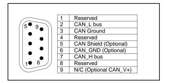
The CAN signals are available via the 9 pin male D-sub connector on the top of the unit. This connector follows the standard D9 configuration. A breakout module (QCI-BO-K) is available to break these signals out to a screw-terminal header.
