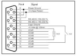
These signals provide power, communications and 3.3v IO (digital and analog).
