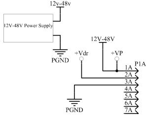
The second configuration, shown right, connects the power supply input (12-48V) to +Vdr (Pins 2A & 2B) through a high power Schottky diode. The high power Schottky diode (60V/6A) keeps the internal driver regenerated power from causing the power supply to shut down and enables the clamp circuit to operate properly.
