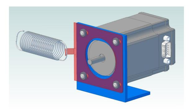
The drawing above shows the tensioning plate as semi-transparent only to allow the mounting plate behind it to be seen. This would normally be made of metal. The fish scale is shown as a spring; it is only present while setting the belt tension. After tightening the screws, the spring/scale is removed. A PDF version of this drawing is included which can be rotated for further information.
