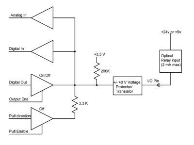
voltage is higher, such as a 5v optical relay or a 24v input to a PLC.
