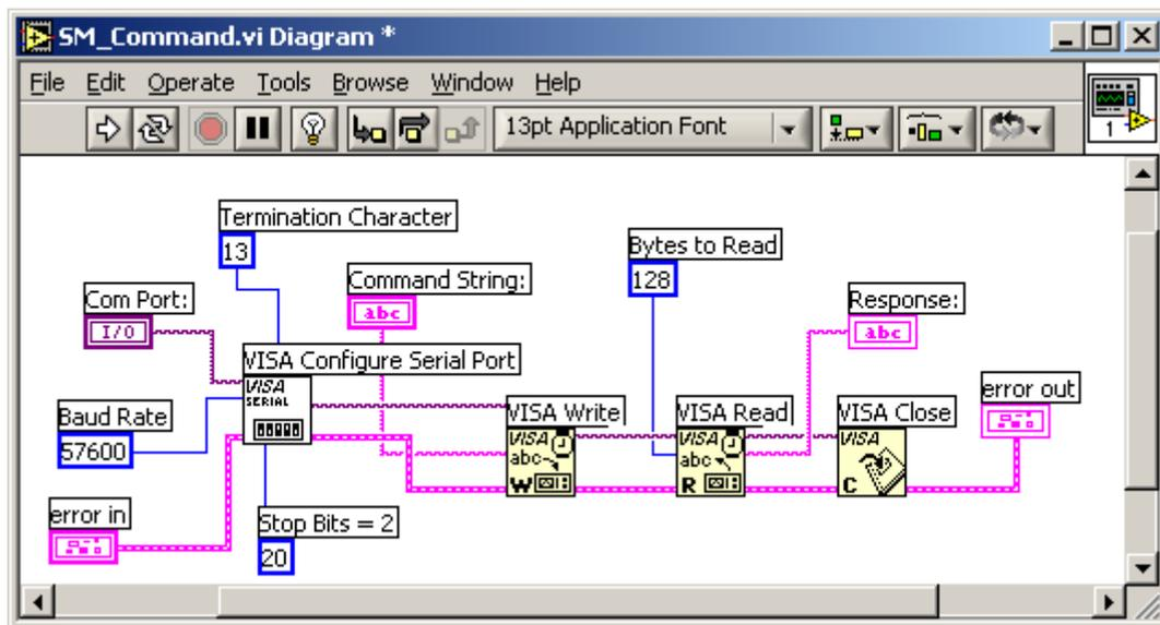
The screen above is the diagram window (panel not shown). Visa Configure Serial Port is the serial communication device, the backbone of the program. Visa Write, Read and Close are functions that enable writing, reading and closing of the COM port. All other items are inputs, outputs and constants labels.
