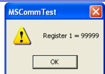
When the 'Test' button is pressed, MSCommTestDlg::OnTest() sets up the COM Port and sends out an LRP command to the device. OnTest() then looks for a returned completion bit before displaying the complete returned data. Once the program is complete, OnTest() sends out an RRG command, which returns the information stored in register 1.
