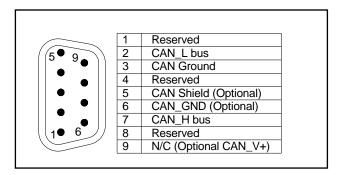
The CAN signals are available via the 9 pin male D-sub connector on the top of the unit. This connector follows the standard D9 configuration. A breakout module (QCI-BO-K) is available to break these signals out to a screw-terminal header.
