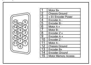
QCI recommends our QCI-C-D15P-D15S-nn (nn = length) cable to interface between the motor and the controller. Note: 01, 02, 04, and 10 foot cables are standard lengths.
