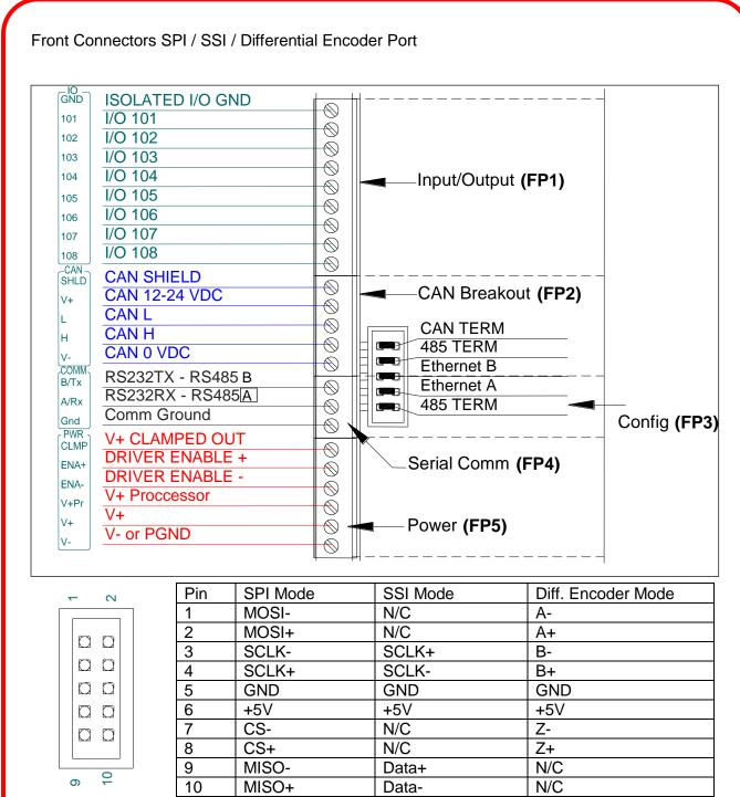
This optional port allows for a differential connection for an SPI port, which is also used for SSI connections, or for use with a differential encoder input. The SSI may be configured for 8 to 31-bit interfaces, binary or Grey code.
