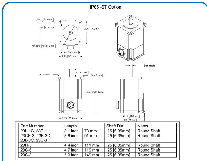
Note: These servo motors are IP65 except front shaft. If not otherwise protecting the front shaft, a Shaft seal (QCI-23M-65) is required for full IP65 (sold separately).
