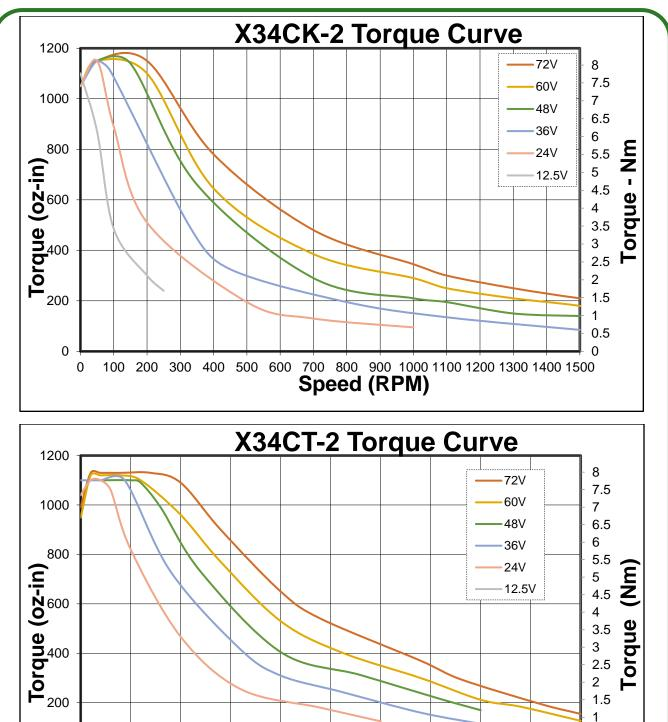
Note: All torque curves taken with 2' power cable; voltage measured entering power cable.
