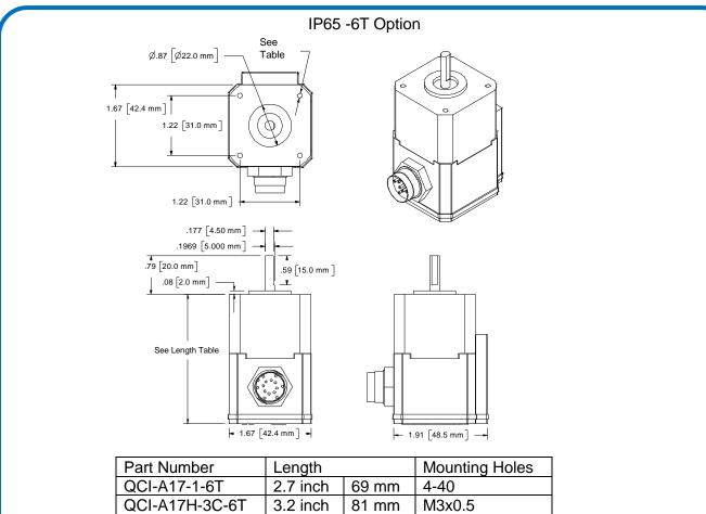
Note: These servo motors are IP65 except front shaft. If not otherwise protecting the front shaft, a Shaft seal (QCI-17M-65) is required for full IP65 (sold separately).
