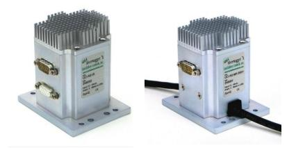
Power, communications, and I/O are accessed through a single DB15 high density interface connector. The interface includes 7 I/O, all of which support both LVTTL and analog signals, and one of which also supports 0 to 10v analog. A hardware drive enable is available as a factory option (Special order). All 7 I/O also have soft configurable pull-up/pull-down resistors, which may also be disabled, for more flexibility
