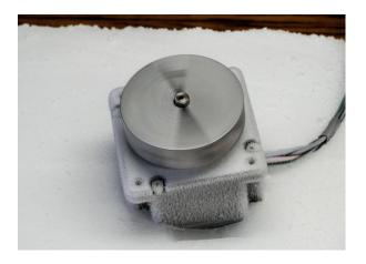
The Mosolver works over a wide range of temperatures. The picture shows a 23 frame Mosolver operating in a block of Dry Ice. For high temperatures, the Mosolver should be able to match the ratings of the motor as well.
