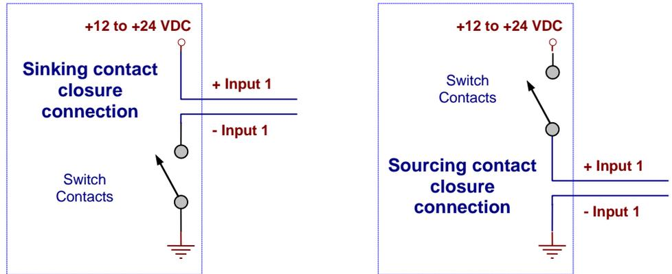
Connecting A Sensor With An Open Collector NPN Or PNP Output To Input #1
