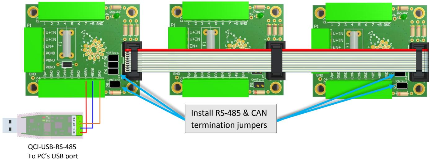
Two ribbon cable options are offered, standard and twisted pair. For short cable runs between breakouts, the standard ribbon cable is acceptable. For longer cable runs or when near noisy environments, the twisted ribbon cable is recommended.
