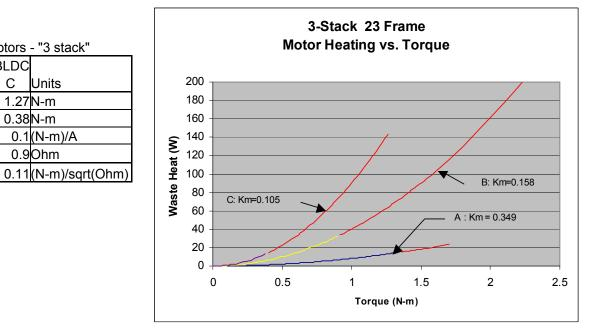
The lower curve is Step motor, A, the middle curve is BLDC motor B, and the upper curve is BLDC motor C. The red portions of each curve represent the motor as it is operated beyond continuous torque rating, but within the peak torque performance rating.
