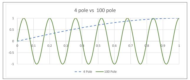
The above graph portrays the normalized flux of a 4-pole motor to a 100-pole motor as the shaft is rotated. The rate of change of the flux (slope) times the number of turns is what produces the backEMF. The current through the winding overcoming the backEMF is what is transformed into the motor mechanical power. The higher the product of backEMF and current, the higher the instantaneous motor power.
